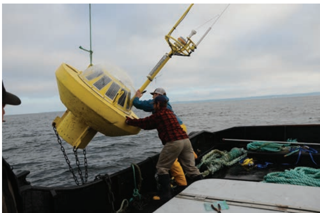
Dr. Bryson Robertson, (in blue jacket) and the boatman launch a WatchMate and TriAXYS wave-measurement buoy near Ucluelet, off the west coast of Vancouver Island, British Columbia. Photo courtesy West Coast Wave Initiative.
