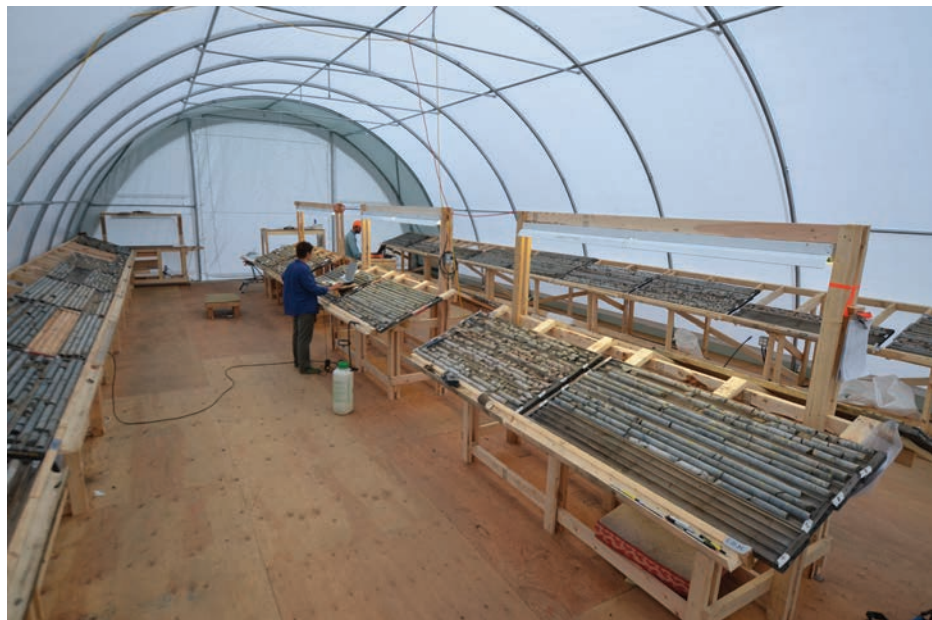
Olga Prikhodko, Red Pine geologist, logs diamond drill core at Wawa Gold Project located 2 km southeast of Wawa, northern Ontario. Photo courtesy Red Pine Exploration Inc.
